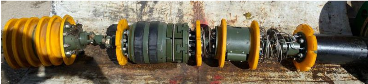
Figure 6: 8" Tethered Abandonment Plug, Post Factory Acceptance Testing
